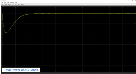
Figure 1.18: Total power of AC loads
